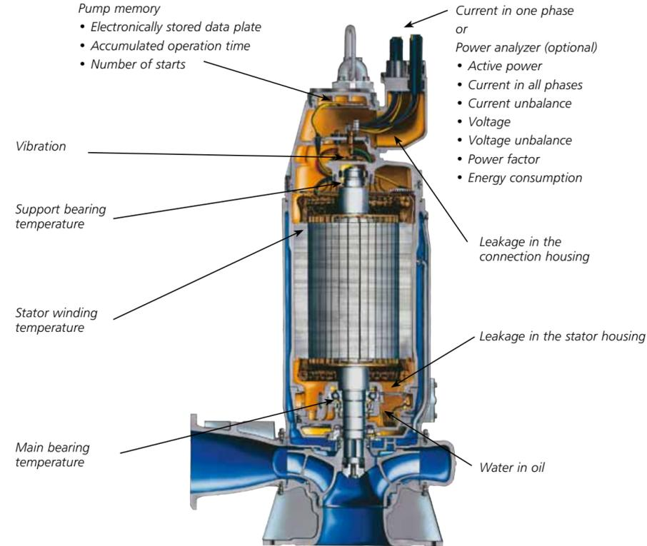
Flygt MAS 711 monitors and stores measurements from the customer's selection of factory-installed sensors. In addition, essential data about the pump useful for installation, servicing and maintenance (stored in the pump memory) is automatically synchronized with the corresponding data in the base unit every two hours.
